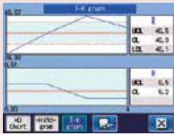
Graphic display of statistical calculation results and X-R control charts
