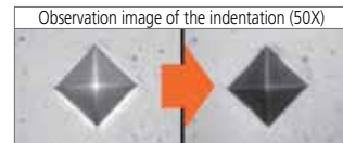
Stray light reduction around the indentation
