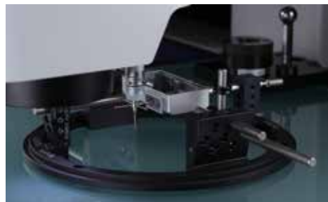
QV Active with optional Opti-fix clamping system
