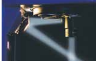
Switchable surface illumination: vertical or oblique
