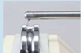
Inner/outer ring contour of a bearing
