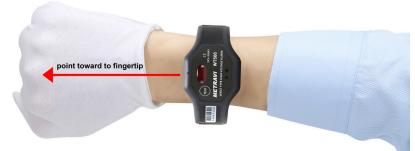
The alarm is to be worn on the wrist of the operator, with the alarm  $\triangle$ symbol pointing towards the direction of the fingertips.
