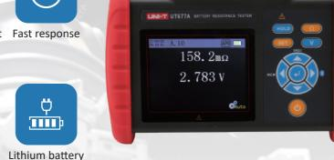
The battery internal resistance tester is a measuring instrument used to measure the internal resistance, voltage, and temperature of rechargeable batteries such as lead-acid batteries and lithium batteries to judge the health status of the battery.
