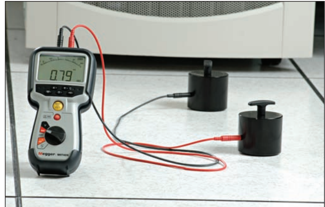
MIT40X shown measuring electrostatic charge in a computer control room.
