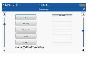
Click to turn on/ off the mic phone, the operator's voice can be recorded, convenient to distinguish the recording location and make records
