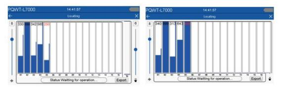
**Locating** which is mainly used to locate the leak points in suspected leakage areas.
