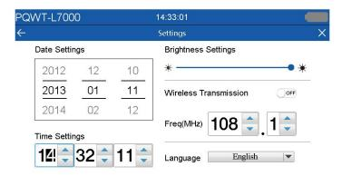
Wireless transmission: It can be received by USING FM radio or mobile phone headphones with FM radio function. It is convenient for multiple people to listen at the
